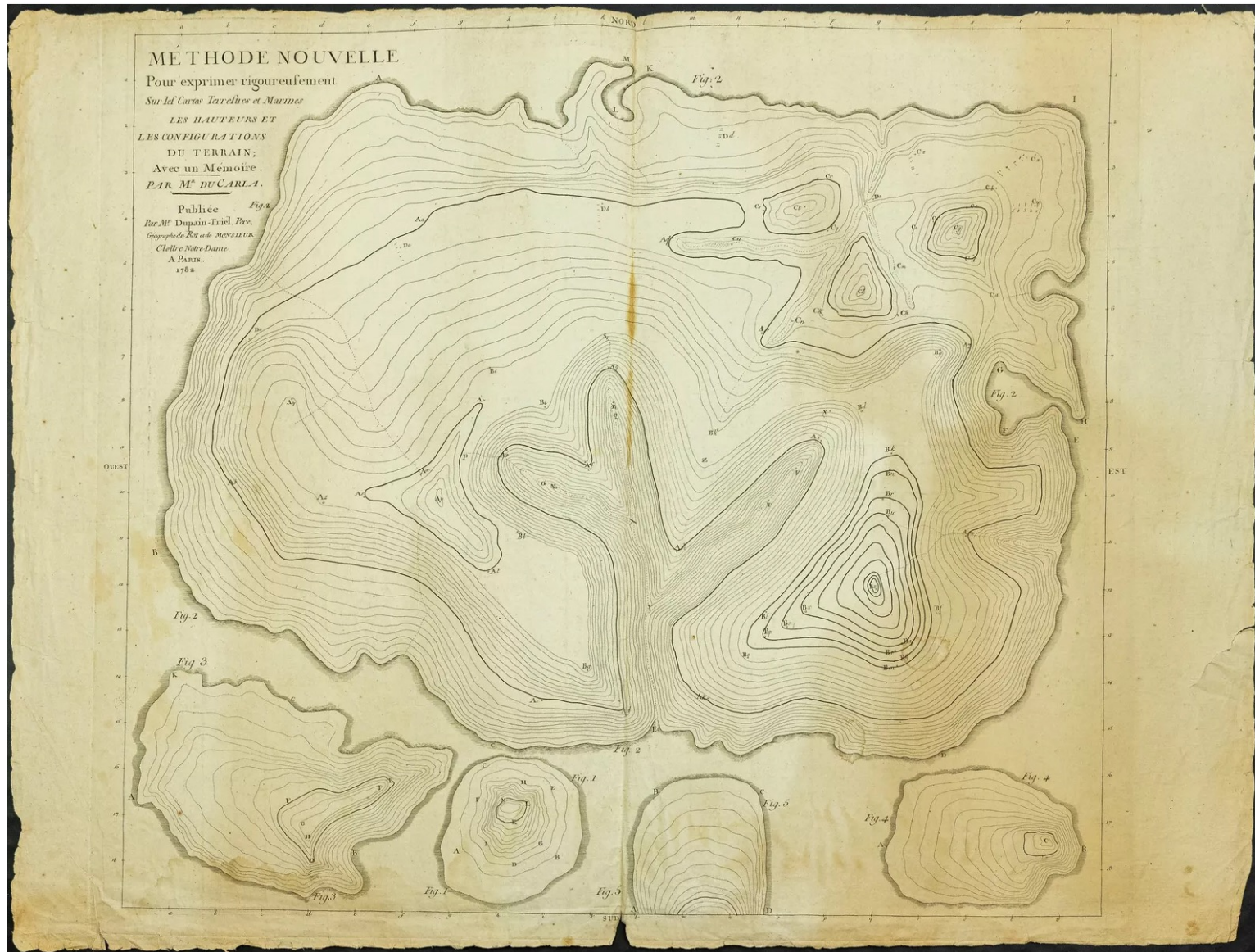
Early topographical map with contour lines (from Marcellin Du Carla-Boniface, Expression des nivellements , Paris, 1782)
