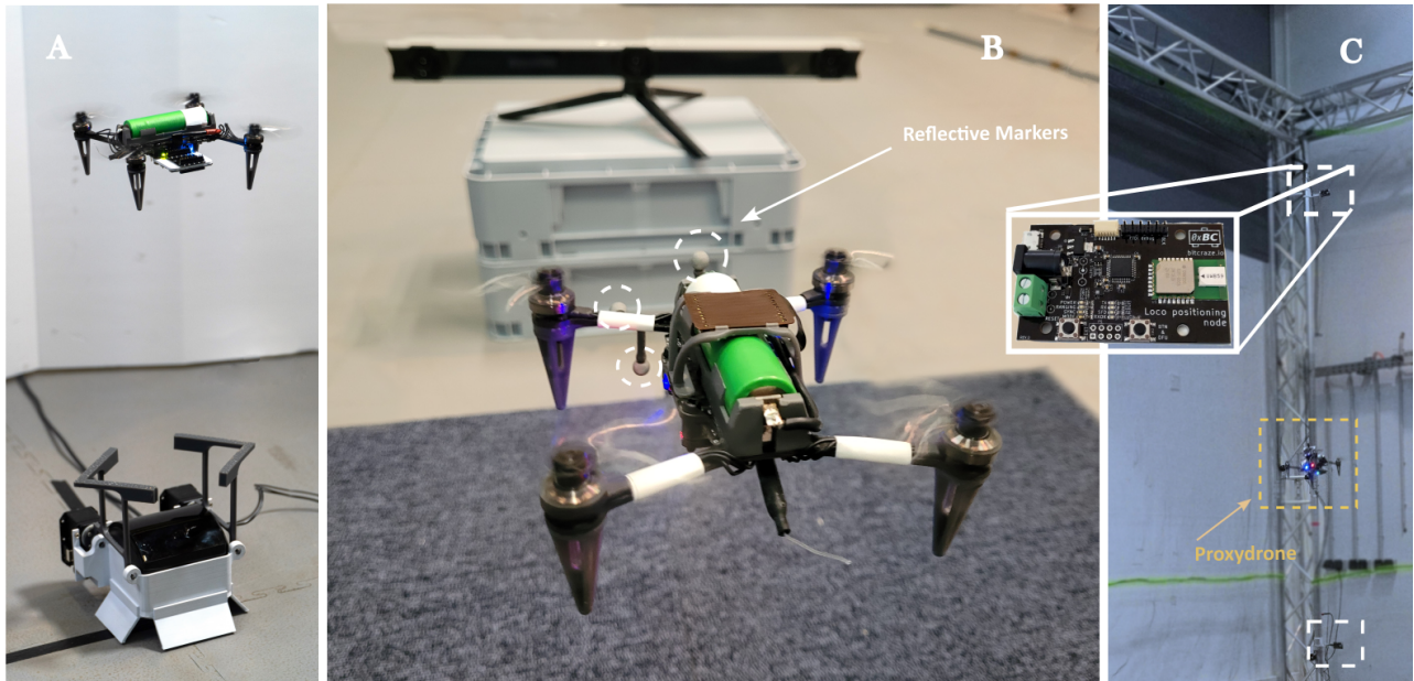
Fig. 5: The composite image encapsulates different positioning estimation technologies approaches for precise docking compared during the landing tests. (A) exhibits the Proxyfly engaging with a lighthouse docking station to perform a precision landing. (B) depicts the Proxyfly in flight. Its movement is tracked by an OptiTrack Trio system. (C) displays the Proxyfly utilizing the Loco Positioning System that operates on UWB technology.
