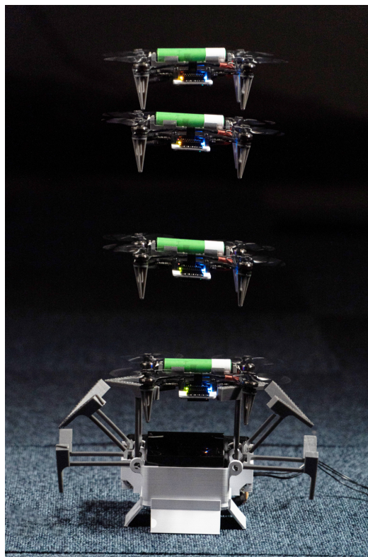
Fig. 1: A high-resolution, time-lapse shooting sequence capturing the autonomous landing of the Proxyflie drone (a.k.a. Proxydrone). The sequence is depicted in different stages: initial alignment with the docking station, followed by a gradual descent and approach with the landing gear extended towards the docking interface, culminating in the drone resting securely upon the docking station, signifying the completion of a successful landing. The supplementary video ( https://tinyurl.com/SpotreturnICUAS24 ) shows 3 successful landings with the Lighthouse-based docking station.
