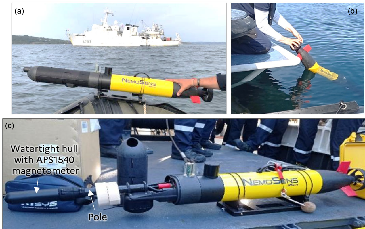
FIGURE 3 NemoSens micro-autonomous underwater vehicle (AUV) (RTSys). (a) AUV ready to dive in front of BH2 Laplace vessel. (b) Launch from the rear platform deck of the hydrographic launch. (c) Watertight hull encapsulating the Applied Physics Systems 1540 vector fluxgate magnetometer tied to the AUV by a pole.
