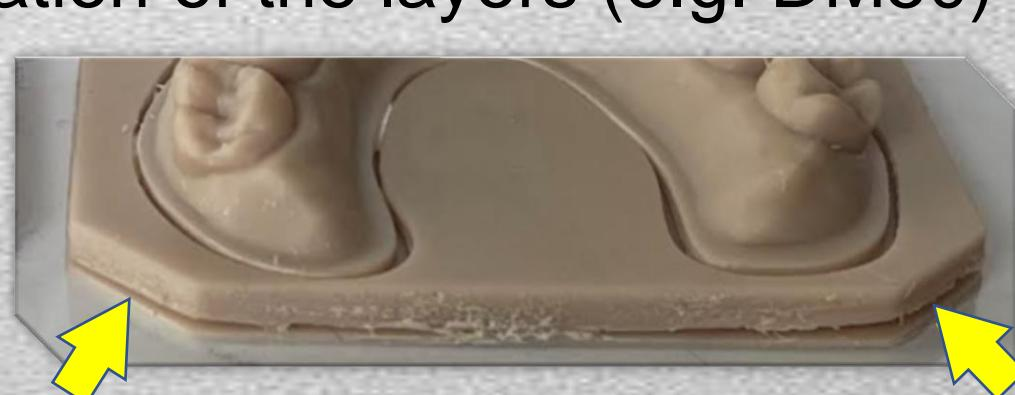
➤ **Pixel smoothening** in the new-gen “optimised LCD” could reduce the closeness with the original STL model
