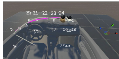
FIGURE 14. Hand motion from points 2-11 in unity software for STA and STB. The predicted hand is shown in white with a white trail and the real hand is brown with a pink trail
