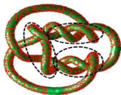
Fig. 1. Model adjustment to a point cloud (green shape adjusted to the red spots). The dashed ellipses delineate topologically complex regions that are hard to fit correctly.
