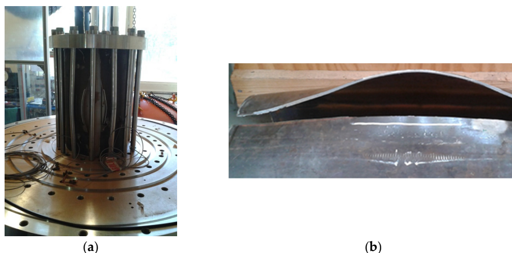
Figure 9. Burst DN 300 pipe section still mounted on the test cell (a) and removed (b).
