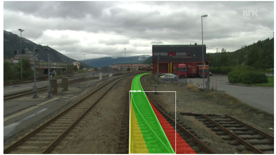
Fig. 11: Late fusion: Incorrect ego track calculation due to (a) missing spline points (b) partially visible merging switch. Green areas=True Positive, Yellow areas=False Negative, Red areas=False Positive. White rectangles represent results of the switch detection network.
