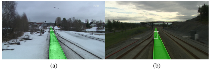
Fig. 12: Positive Examples of ego track detection for (a) Early Fusion algorithm (b) Late Fusion algorithm. color meanings as in Figure 11.
