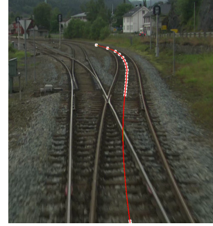
Fig. 9: Late fusion: Interpolated centerline using spline interpolation shown as red line. For reference spline points used for the interpolation are shown as well as white dots.
