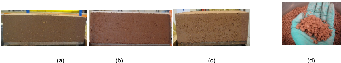
Figure 3. Blocks made with 5% cement+ SCBA with 9% (a), 10% (b) and 11% (c) water content added, respectively (5CB9, 5CB10 and 5CB11) and pelleted mixture in the small pan mixer (d).
