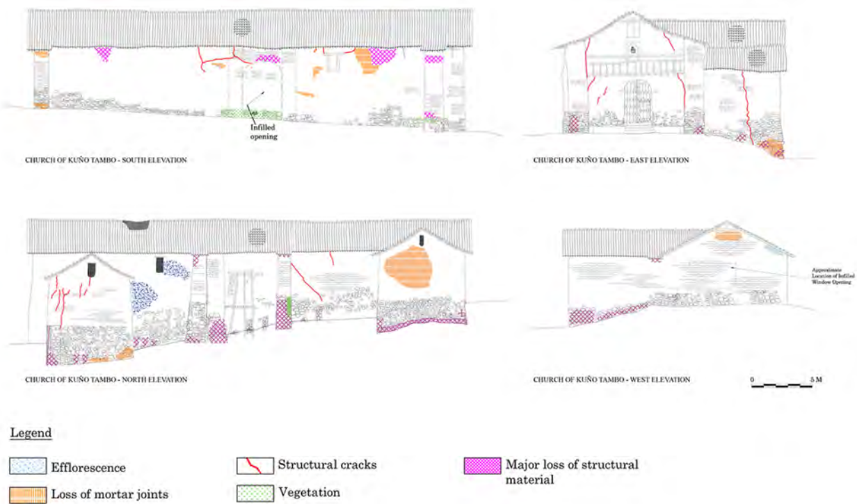
Fig. 3 Damage maps in each facade [5].
