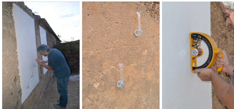
Figure 1. Karsten tubes test in commercial renderings and ancient renderings; pendulum hammer test.
