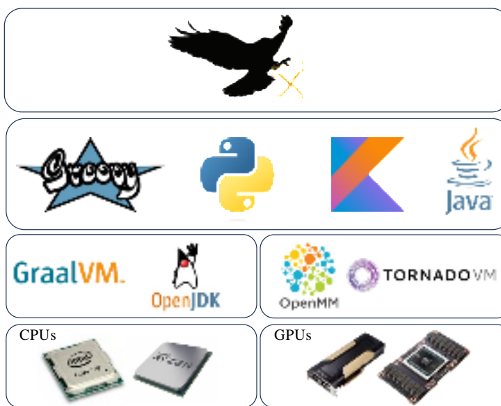
Figure 1. An overview of Force Field X. The second row shows languages that are compatible with FFX. The third row represents the platforms that execute FFX on CPU cores on the left and coprocessors on the right. The final row indicates the CPU and GPU hardware that FFX can perform calculations on.
