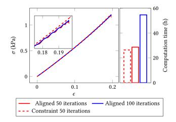
Figure 6: Left: Stress-strain curves for the tilted scenario simulated with an aligned mesh, both with and without the inextensibility constraint. The unconstrained calculations were made with 50 (—) and 100 (—) non-linear iterations. The constrained version (---) used at most 50 nonlinear iterations. Inset: due to poor conditioning, unconstrained results tend to oscillate. Right: with the inextensibility constraint, oscillation-free solutions are computed at much lower cost.
