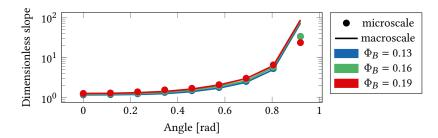
Figure 11: Comparison between slopes of the stress-strain curves of the macroscale model and the microscale model in traction scenarios with barbs oriented at different angles. The slopes are nondimensionalized through scaling by the Young modulus of the barbules in the microscale model  $E_b$ . Comparison is done using the measured barb density  $\Phi_B = 0.16$ , as well as the two extreme values of the error range  $\pm 0.03$ .
