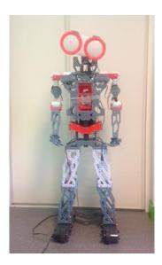
Figure 1. Meccanoid G15KS robot.
