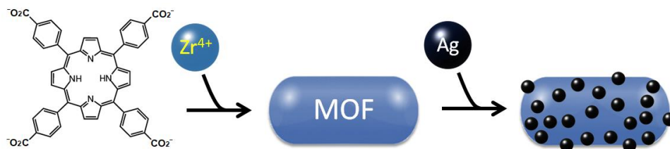
Figure 16. Scheme showing the conceptual design of the nanohybrid ZPM@Ag. The MOFs were prepared from H_2TCPP and ZrCl_4 with benzoic acid in DMF under solvothermal conditions. Then, the Ag NPs were added to the MOFs upon mixing them with AgNO_3 in water at 80^\circ C . 81
