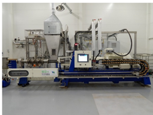
Figure 1. Extruder Clextral Evolum EV 53 for polyphenol extrusion-extraction.
