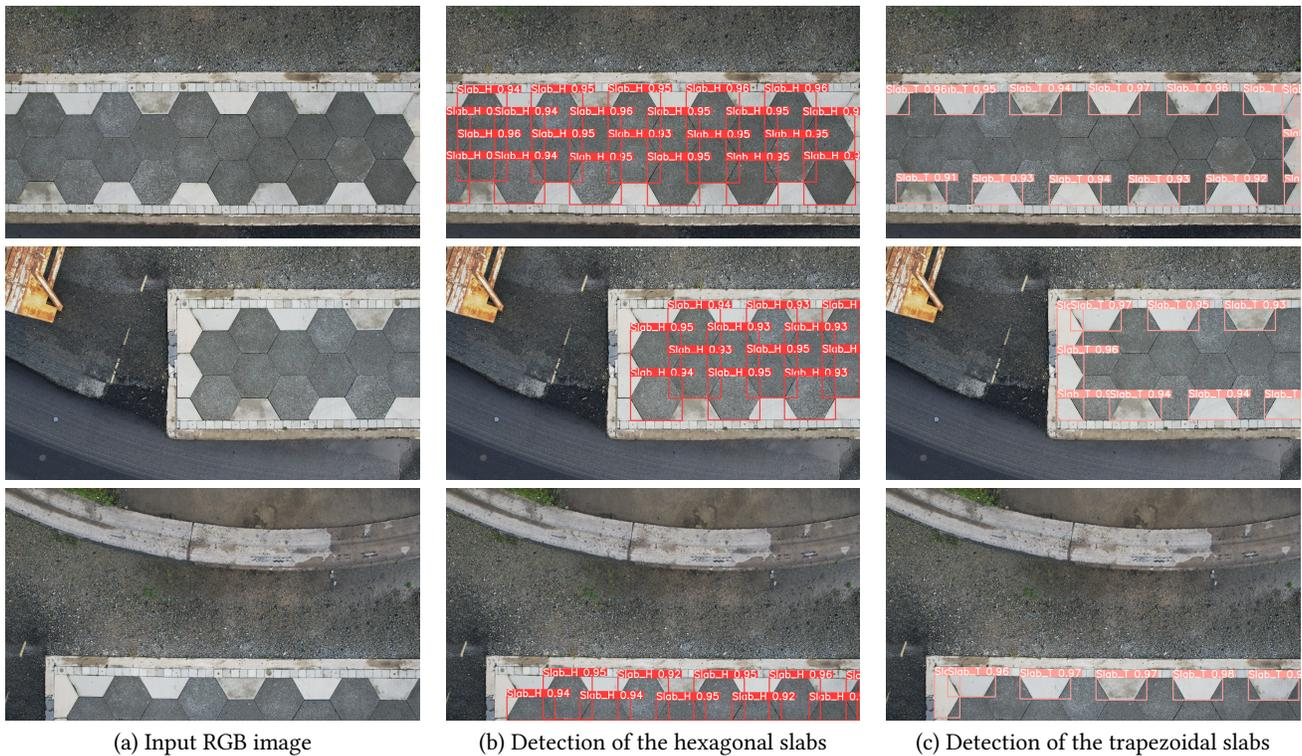
Figure 11: Indicative outputs of the YOLOv8s model.
