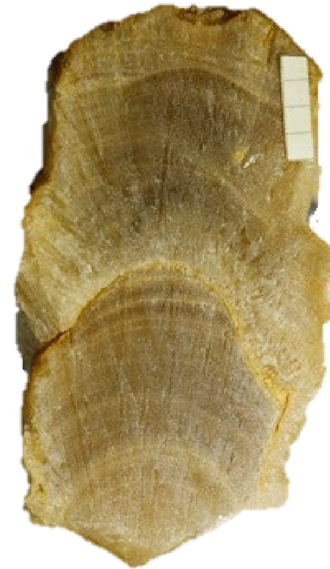
Samples taken from the cave : (A) speleothem D003_4_1, (B) and (C) paleomagnetism cubes.
