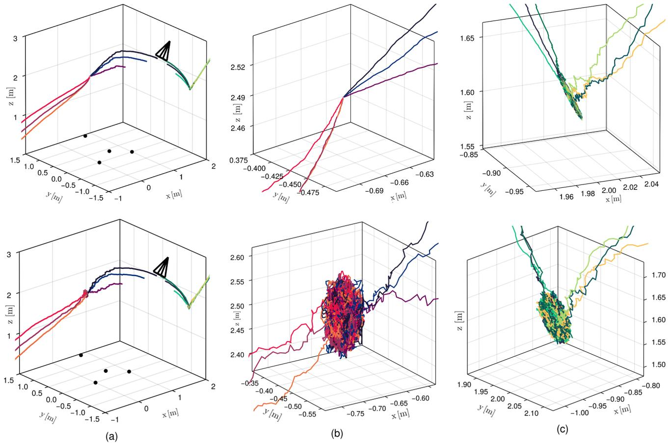
Fig. 10. Selection of 12 simulations with noise on  $\mathbf{Z}$  only on top row and with simultaneous noise on  $s$  and  $\mathbf{Z}$  on bottom row. (a): Trajectories overview, where 6 of the initial poses were chosen around each saddle point. (b)-(c): Zoom-in at the desired pose and local minimum, respectively.
