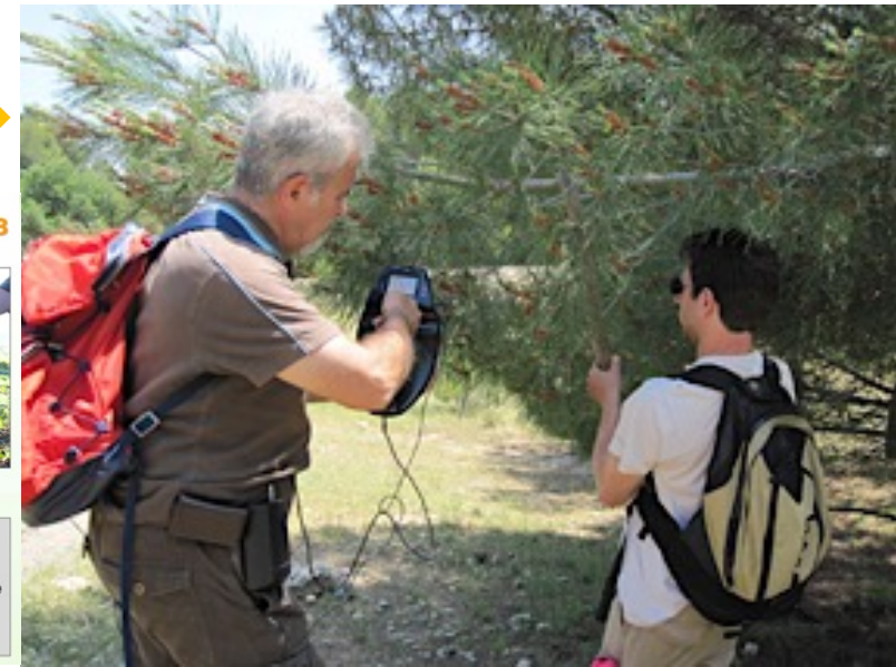
Non-destructive measurements of plant compounds with a portative fluorimeter
