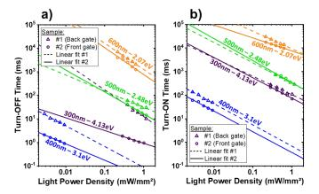
Fig. 3. a) Turn-OFF and b) Turn-ON time for both samples as function of the illumination power density for different wavelengths. Open triangles markers and open round markers stand for sample #1 and #2 respectively, measured data point, whereas dashed (#1) and solid (#2) lines are power law fits with an exponent ranging between 0.5 and 1.12 for each wavelength value.
