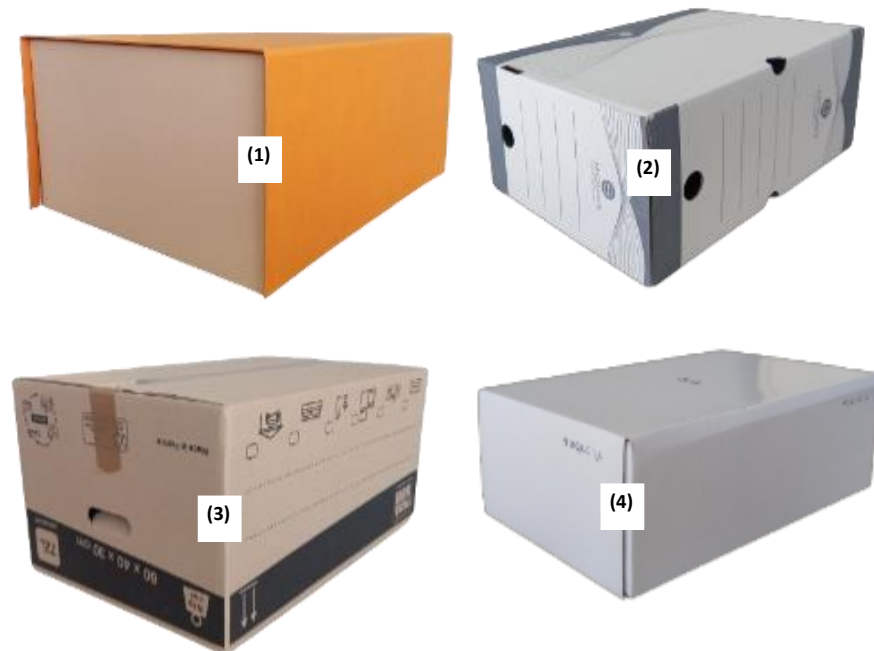
Figure 2. Different cardboard raw materials: (a) sample #1 (2.2 mm thickness), (b) sample #2 (2.15 mm), (c) sample #3 (3.6 mm), (d) sample #4 (1.7 mm).
