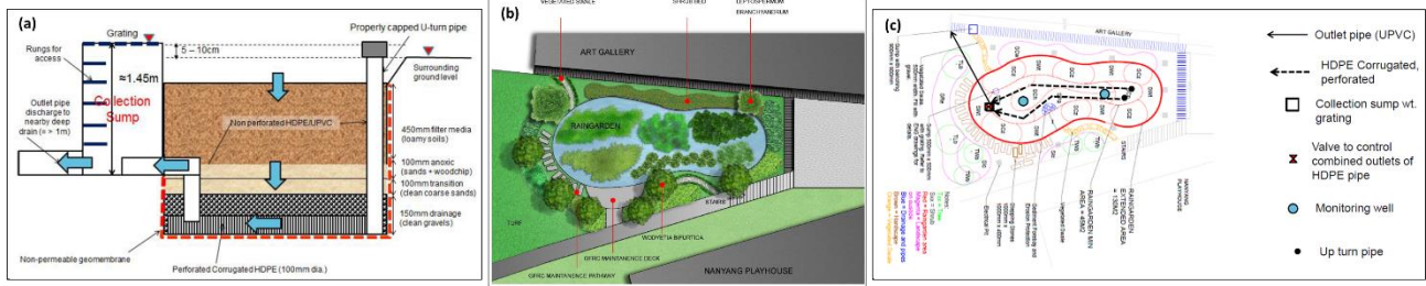
Figure 1. (a) shows the cross-section of the Rain Garden monitored by the low-cost sensor monitoring system; (b) and (c) shows the main catchment area and the theoretical water flow for this Rain Garden (Credit: Kim Irvine, AECOM).
