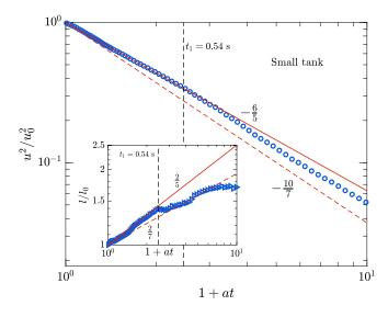
FIG. 2. Decay of the squared velocity fluctuations  $u^2$  as a function of the rescaled time 1 + at (water). The solid line corresponds to a power law defined as  $(1 + at)^{-6/5}$  (Saffman) and the dashed line represents the power law  $(1 + at)^{-10/7}$  (Batchelor). Inset: time evolution of the integral scale l. The solid line represents the power law  $(1 + at)^{2/5}$  (Saffman) and the dashed line  $(1 + at)^{2/7}$  (Batchelor).
