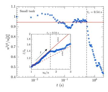
FIG. 1. Time evolution of Saffman invariant  $u^2 l^3$  using water as working fluid. The solid line represents the mean value of the invariant up to  $t_1 = 0.54$  s. Inset:  $l/l_0$  as a function of  $u_0/u$ . The equation of the solid line is  $y = (u_0/u)^{2/3}$ (Saffman) and the dashed line is  $y = (u_0/u)^{2/5}$  (Batchelor). The black arrow represents the direction of time and the dashed line gives the time  $t_1$  after which  $u^2 l^3$  decreases significantly.
