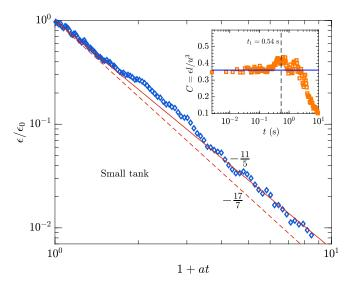
FIG. 3. Decay of the energy dissipation rate  $\epsilon$  as a function of the rescaled time 1+at, with water as working fluid. The solid line represents  $(1 + at)^{-11/5}$  (Saffman) and the dashed line  $(1 + at)^{-17/7}$  (Batchelor). The initial value of the dissipation rate is  $\epsilon_0 = 2.1 \times 10^{-3} \text{ m}^2/\text{s}^3$ . Inset: time evolution of the constant C measured from the ratio  $\epsilon l/u^3$ . The solid line represents the mean value of C for  $t \leq t_1$ .
