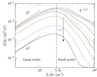
FIG. 5. Decay of the energy spectrum in the large reservoir. The vertical dashed line corresponds to the initial inverse integral length  $1/l_0$  separating the large and small scales. Here, t = 0, 0.09, 3.66, 5.96, 15.83, 42.01, and 104.99 s.
