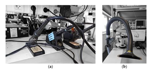
Figure 1. (a) desoldering station, (b) fume extractor.
