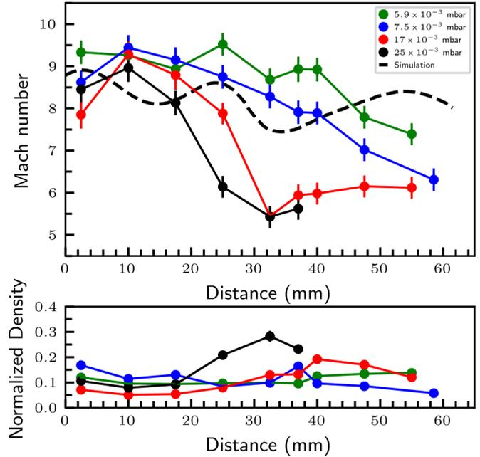
FIG. 4. The measured Mach number distribution (top) and density distribution (bottom) along the jet core for  $P_0 = 80$  mbar and different background pressures. The calculated Mach number along the gas jet is shown as a dashed line.
