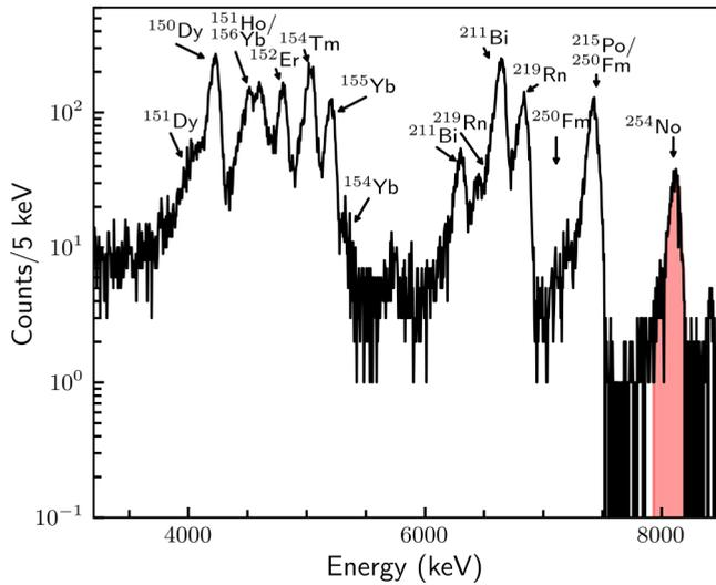
FIG. 6. Alpha spectrum of the nuclei observed during the online experiment using the silicon detector at high voltage as described in the text. The decay chains of  $^{155}\text{Yb}$ ,  $^{254}\text{No}$ , and  $^{223}\text{Ra}$  are shown. The red shading indicates the energy gate used for cutting the data on  $^{254}\text{No}$ .
