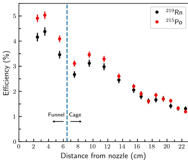
FIG. 7. Offline transport efficiency of the  $^{219}\text{Rn}$  and  $^{215}\text{Po}$  daughters of a  $^{223}\text{Ra}$  recoil source as a function of source distance from the nozzle. The recoil source was mounted on an adjustable rod following the central axis of the JetRIS gas cell.
