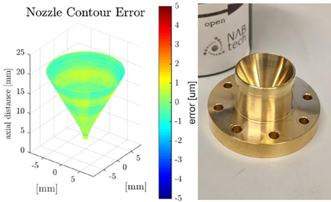
FIG. 3. Picture of the brass low- $P_0$  nozzle (right) with a 3D-visualization of the contour error (left). The error is the contour deviation between machined and calculated contour and is measured with a Werth HA 400 CMM machine in combination with a Fiber-Probe for more than 55 000 points.
