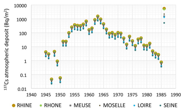
Figure 4. Atmospheric deposits of ^{137}\text{Cs} (Bq/m 2 ) reconstructed from Ref. 26 over the period 1945–1986 for the Loire, Meuse, Moselle, Rhine, Rhone and Seine catchments upstream the core sampling sites.
