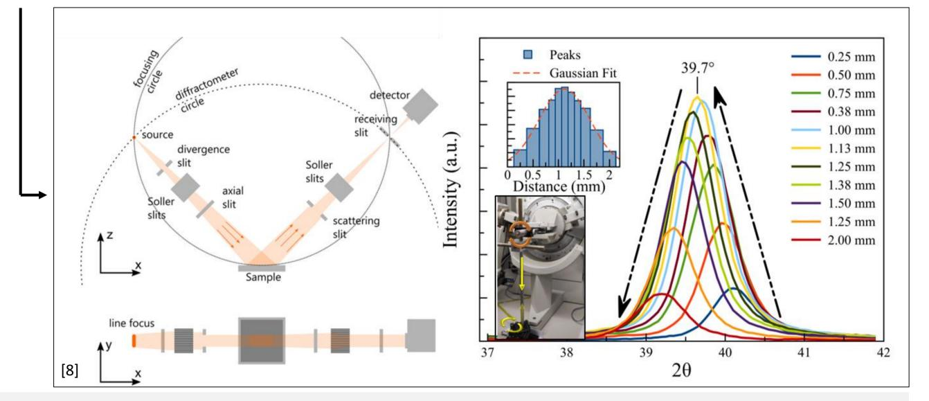
XRD signals were enhanced with a new holder design and understanding the fundamentals of XRD. Yet, peaks were still weak for all samples. What was the next problem?
