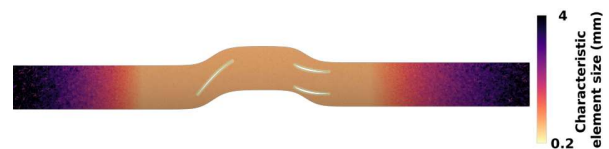
Figure 2: Characteristic size of the elements in millimeters. The reference value for the refined area is 0.8 mm. The mesh is progressively coarsened in order to limit acoustic reflections.
