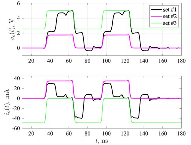
Fig. 3. Training waveforms: transient responses of the example device loaded by three different distributed or lumped loads different from the one considered for validation. Set #1: transmission line with  $Z_0 = 75\Omega$  and  $T_d = 5$  ns; set #2: shunt connection between a  $50\Omega$  resistor and a  $10$  pF capacitor; set #3:  $50\Omega$  in series with the power supply battery
