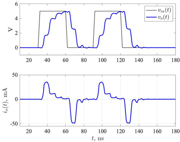
Fig. 2. Test waveforms: transient responses of the example device driven by a “010100” bit stream and loaded by an interconnect with  $Z_0 = 50\Omega$  characteristic impedance and  $T_d = 3$  ns delay.
