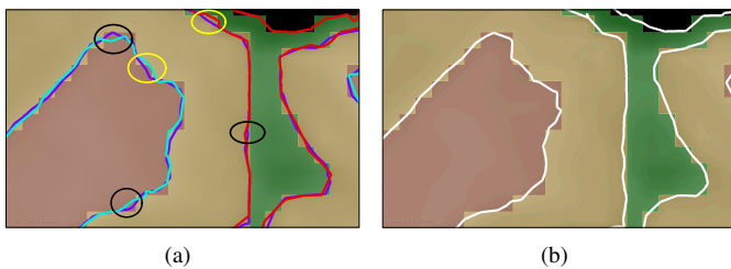
Fig. 16. Examples of the reconstruction of all 3 segments by CGAL 3D Mesh Generation : (a) ROIs independently reconstructed (the color matching of the surfaces are: orange for cerebral spinal fluid, white for white matter and green for gray matter) showing overlaps and empty spaces (respectively in yellow and black); (b) All ROIs at once, in one mesh, without tissue differentiation.
