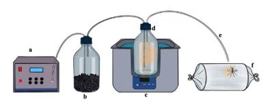
**Figure 1**: Schematic set-up of the behavioral assay (a: stimulus controller; b: gas washing bottle containing activated charcoal; c: water bath; d: sample bottle for insecticide or control solution; e: PTFE tubing; f: cage containing one mosquito female).
