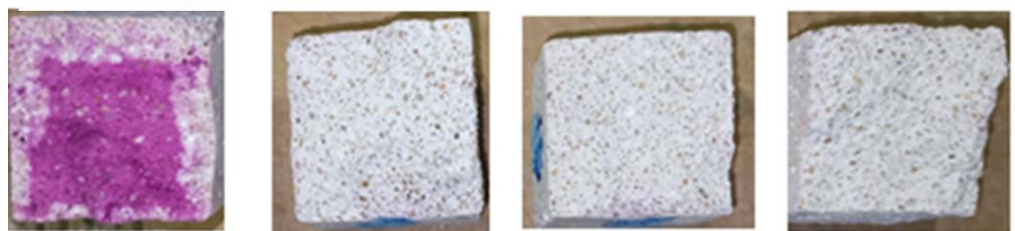
Figure 16. Image of SS-PCM composite mortars ( 4 \times 4 \text{ cm}^2 ) carbonated at 3% \text{CO}_2 chamber ( 20 \text{ }^\circ\text{C} , 65% RH).
