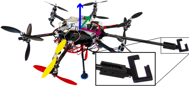
Fig. 2. OMAV platform with hook for the controlled shaking of trees. The body frame of OMAV is indicated with \mathcal{F}_B , with the colored propellers mounted on the arm along the body y -axis. A zoom-in of the hook better shows its details.
