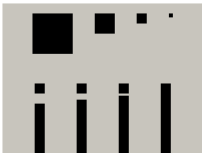
Fig. 2: Target geometry for validation of the fictitious physical field. Black region represents solid \gamma = 0 and white region represents fluid \gamma = 1 . Every boundary is considered as \Gamma = \Gamma_T where T = 0 .
