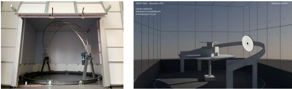
Fig. 11. Mechanical sun within the artificial sky and a computed simulation of a model within the cubic shape of our sun-sky simulator
