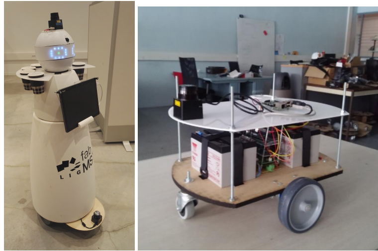
Figure 8. Left: RobAIR mobile robot. Right: RobAIR base.
