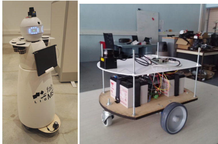
Figure 8. Left: RobAIR mobile robot. Right: RobAIR base.
