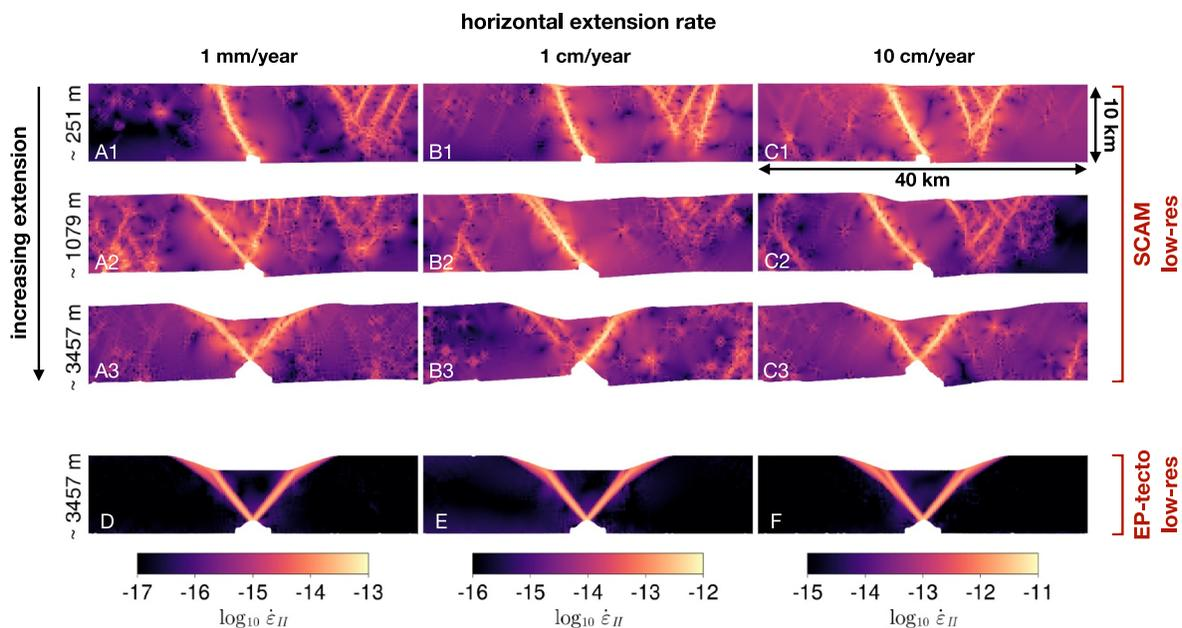
**Figure 15.** Numerical simulation of about 3.5 km of extension of a 10-km thick brittle plate, at varying rates (columns). Snapshots of the second invariant of strain rate at different amounts of finite extension (shown on the left), for a brittle plate governed by a–c the SCAM flow law, and d–f the EP-tecto rheology. The model resolution has been reduced compared to Figure 13 to reach greater amounts of finite extension in reasonable time.
