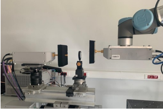
Fig. 5. Collaborative robot measuring the field produced by a GOLA.
