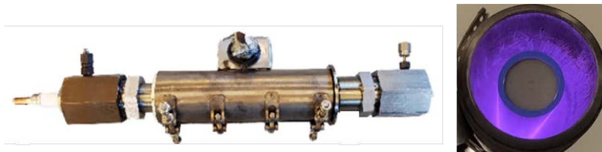
Figure 1. (LEFT) The Catalytic Low Temperature Plasma (C-LTP) reactor system developed in this research project for the reformation of methane. (RIGHT) C-LTP reactor cross section depicting atmospheric low temperature plasma formation in the gas gap.
