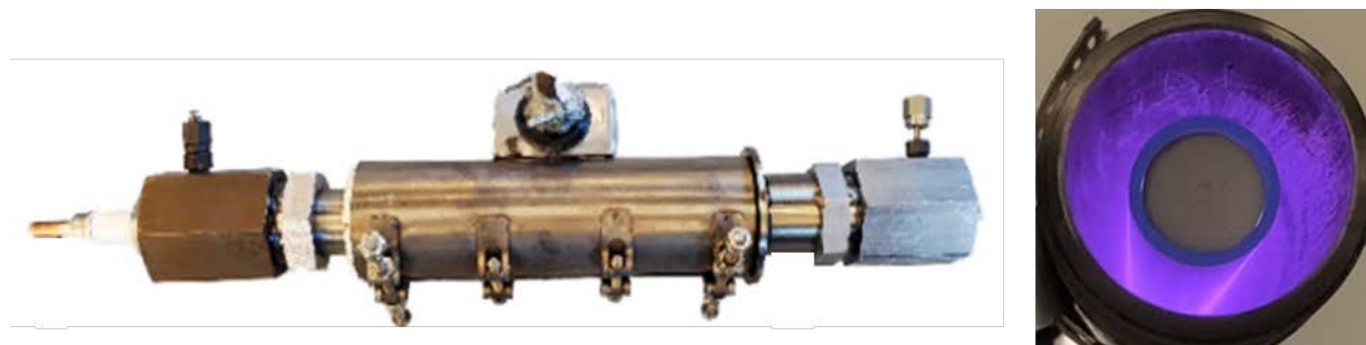
Figure 1. (LEFT) The Catalytic Low Temperature Plasma (C-LTP) reactor system developed in this research project for the reformation of methane. (RIGHT) C-LTP reactor cross section depicting atmospheric low temperature plasma formation in the gas gap.
