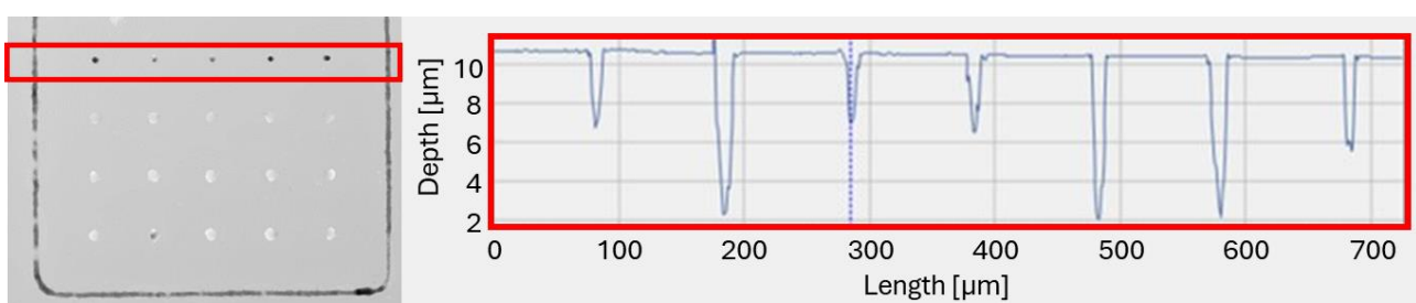
Interferometric imaging of trenches made on glass at different laser powers.
