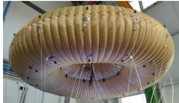
Fig. 21. IS demonstrator under excitation (free-free).
