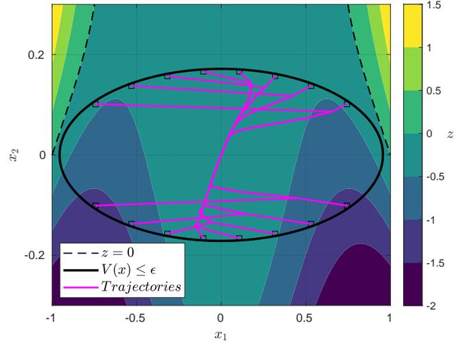
Fig. 1: Contour plot of  $z = v_1 (x_1^2 + x_2)^2 - v_1 x_1^2 - x_2^2 Q$  illustrating region where  $z < 0$ , a sublevel set of the Lyapunov function  $V(x) \leq \epsilon$  included in the region where  $z < 0$ , and closed-loop trajectories.
