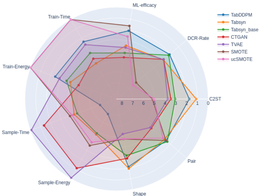
Figure 5: Radar chart of the extensive experiment showing optimized model’s average ranking on all datasets according to C2ST, DCR-Rate, ML-Efficacy, column-wise similarity (“Shape”), pair-wise correlation (“Pair”), training and sampling time and energy costs. For all models except “Tabsyn_base”, which refers to the model using its default hyperparameters, the training costs include both tuning and gradient descent.
