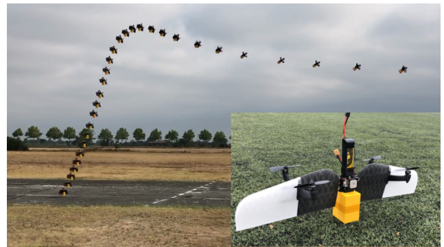
Fig. 1: Sequential imagery of vertical take-off and transition in a test flight and vehicle ready for IMAV competition.
