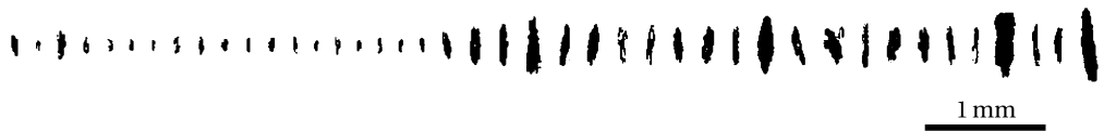
(d) Particles in the wind tunnel, 79 μm median mass diameter, 3.2 gm -3 ice water content and -15 °C air temperature
