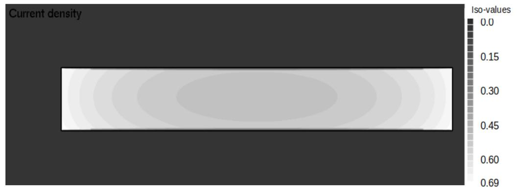
Figure 3. Current density in one branch in units of mA/μm<sup>2</sup> when the total current is 1 mA.
