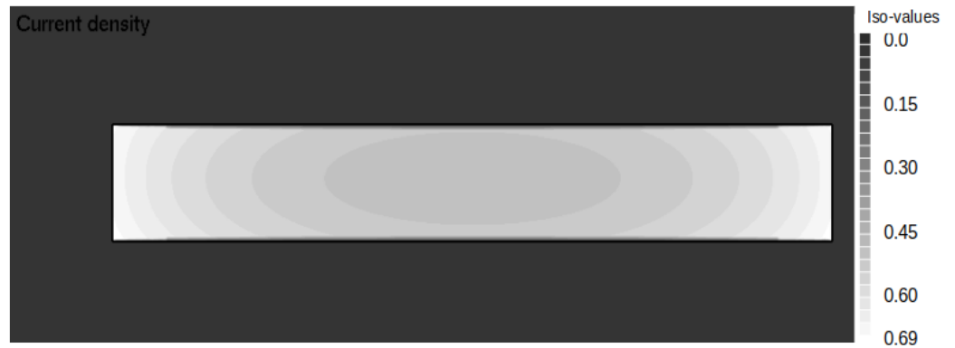
Figure 3. Current density in one branch in units of mA/μm 2 when the total current is 1 mA.
