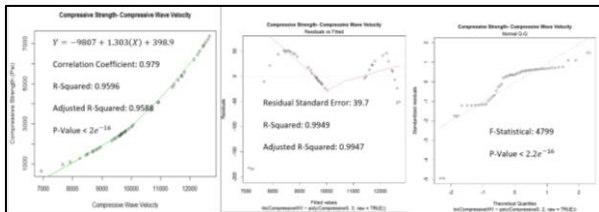
Fig 6: Compressive strength-compressive wave velocity: Regression, residual and normal Q-Q plot
